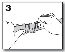
For longer kits, join multiple lengths of guttering using the supplied union(s) by clipping in, ensuring 2 brackets are first slid onto the larger length attached to the stop end outlet and a bracket after each union. Please refer to step 3 for a note regarding the seals.
