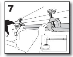
Fine-tune guttering position. It is normal for a rigid downpipe to hang slightly to one side. Horizontal positioning of the brackets may also be adjusted for best effect. To avoid sagging don't place the brackets at the very ends of the gutter.
