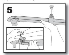
Place the gutter and clamps to the roof edge so gutter is suitably positioned, supporting the gutter as needed whilst nipping up the brackets enough to secure the gutter - **do not overtighten**.
