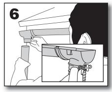
Slide downpipe onto stop-end outlet. For flexible downpipes, the pipe needs to go to the very top, widest part of the outlet and tightened by the clamp key, see inset diagram.
