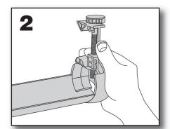
Slide two brackets onto guttering to a suitable distance, between 30cm and 60cm (12" to 24") from each end, with the V clamps facing the rear. It is recommended that brackets are placed roughly 1.2m (4ft) apart, but adjust as necessary.
